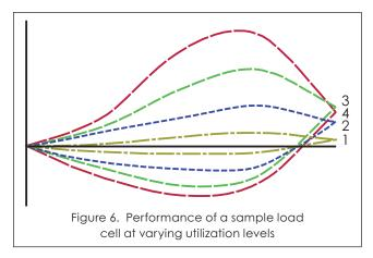
Figure 6 represents the combined error performance of a sample load cell with a rated capacity of 500 kg. The cell has been measured with a utilization of 20% (1), 40% (2), 60% (3) and 80% (4) of the rated capacity.
