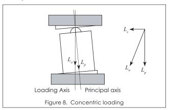
Inclined loading effects should be considered for compression type cells only. Because of bending effects in the column, single column load cells are more sensitive than multiple column cells.
