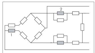
Figure 10. Offset (1) and span (2) temperature compensation. The modulus resistors have a fixed resistance value for a certain load cell model and are being shunted with a so called modulus parallel resistor to obtain specific values
