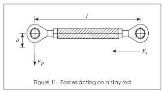
Stay rods are used if major load movement is anticipated, for example in weighbridges or vessels with an agitator. Stay rods are installed horizontally and should not transfer any forces to the vessel or platform. However, because of the inherent load cell deflection, errors are unavoidable. The following
