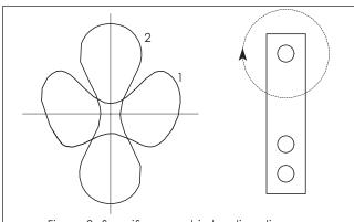
Figure 9. Specific eccentric loading diagram of a bending beam (1) and shear beam (2) type load cell, showing the error experienced at defined eccentric angular positions
